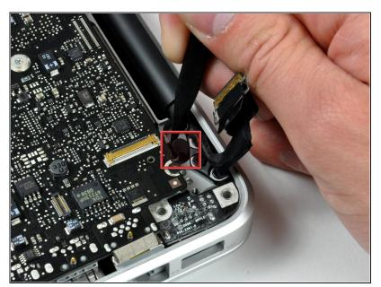
Use the tip of a spudger to release the microphone from the upper case.
