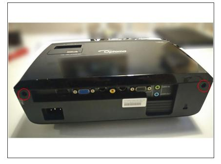
Turn the projector over. Then unscrew the two screws on each side of the back of the projector (circled).
