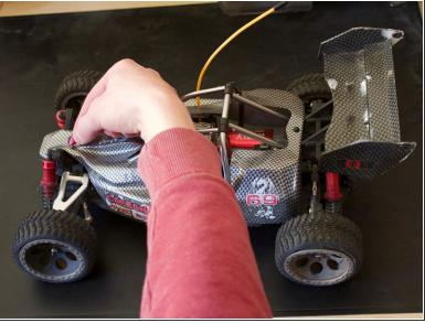
(i) TIP: if you remove the cladding more often (for example, for thorough cleaning), it may be helpful to provide the splints with some insulating tape, so the use of tools is unnecessary
