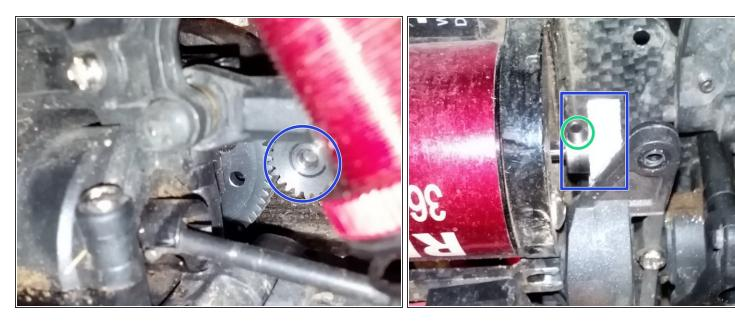
When pushing the new part onto the shaft, please note that it has a flattened side. At this the grub screw (marked in green) should rest.
