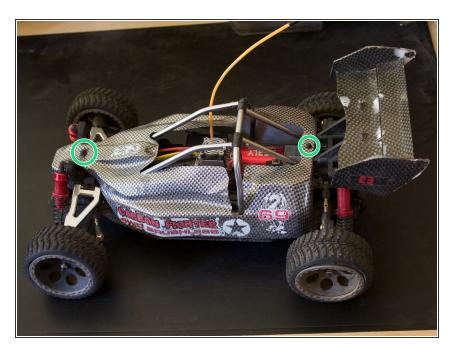
These two pins must be removed.
