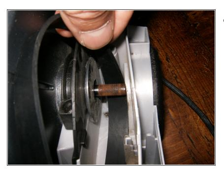
next place the new belt on the motor drive first, then the brush.
