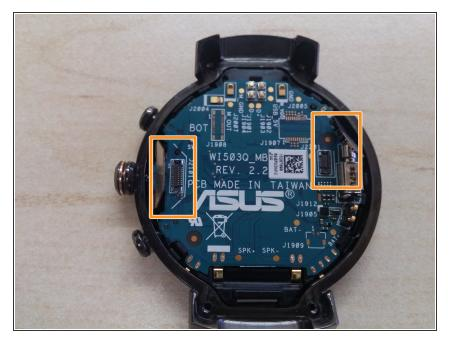
Remove ribbons connected to the board
