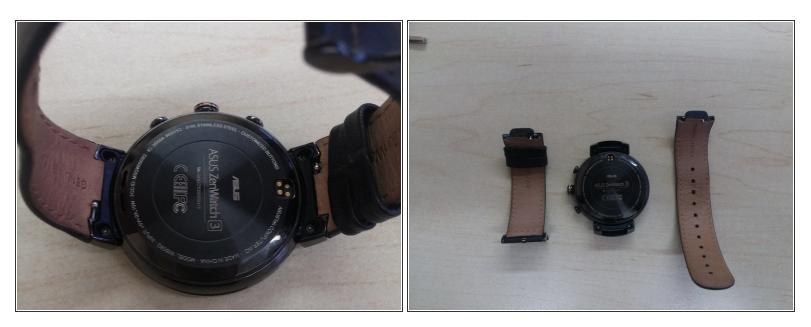
• Remove pins securing the band
