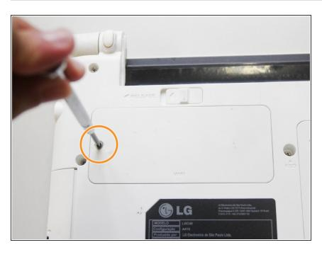
With the notebook upside down, locate the WiFi module cover and unscrew the philips screw.
