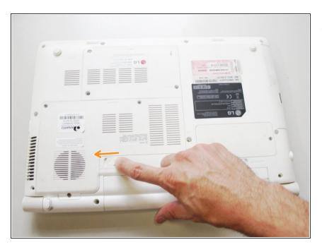
Slide the unlock key in the indicated direction to unlock the battery
