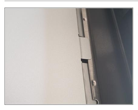
When you re assemble the outer case make sure the tabs on the front go either side of the front.
