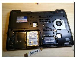
remove the big cover, removing 3 screws
