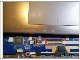
now turn the laptop again and use a spudger te remove the upper case with the keyboard attached to it.
