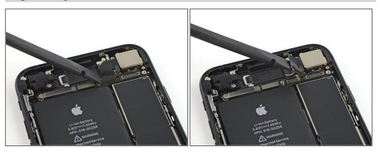
Use the flat end of a spudger to disconnect the rear-facing camera connector.
