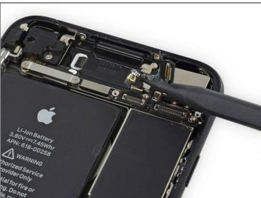
• Use the pointed end of a spudger to pry up and disconnect the antenna bus connector, just left of the rear camera module.
