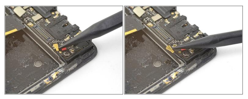
Slide the point of a spudger underneath the antenna interconnect cable and pry up, disconnecting it from the daughterboard.
