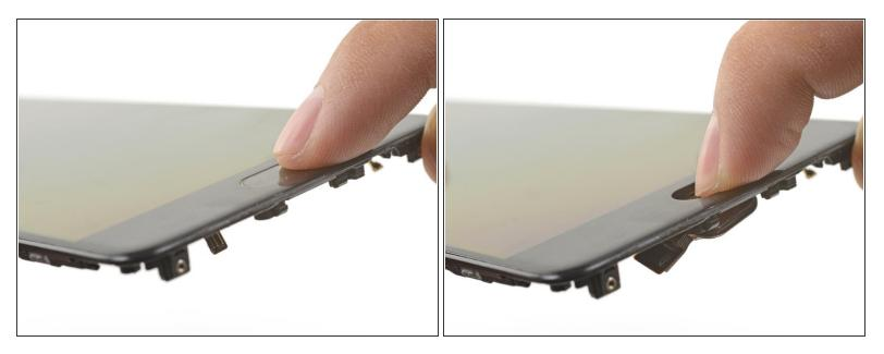
• Use a finger and firmly push on the fingerprint scanner from the front of the display until the fingerprint scanner dislodges from its recess.
