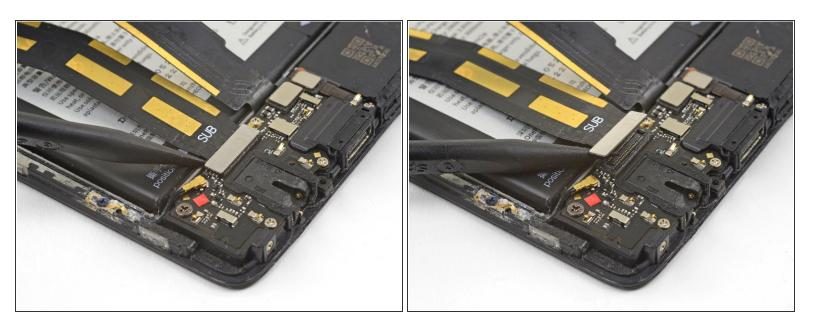
Use the point of a spudger to pry up and disconnect the interconnect flex cable from the daughterboard, which is located below the battery.
