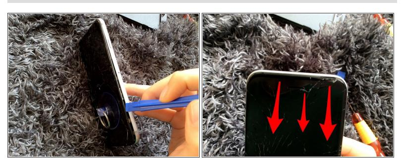
Alice stick with the screen out of the three sides, gently pull down the screen, and then you can open the screen.
