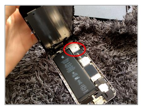
To maintain the 90-degree position, remove the five screws shown in the circle, be sure to place in accordance with the original location.
