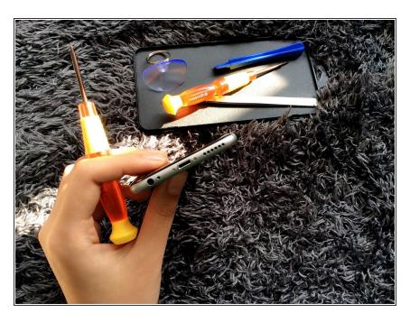
Shut down the phone and remove the bottom screw
