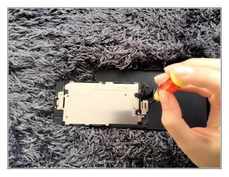
Remove the cover of the front camera and the earpiece. Screw position is still in the distance without interference as the original place away.
