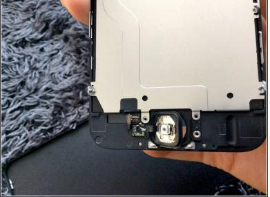
Remove the home key and metal, around home button is glue, if the computer is open, on the cooling mouth blowing, can push it behind To reassemble your device, follow these instructions in reverse order.
