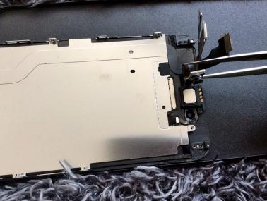
Unplug the front camera and remove the handset
