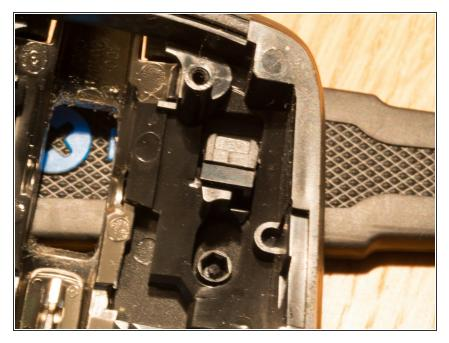
• After the four screws are removed, the top and the bottom part can be easily taken apart. In the top part the grove that was made by the clicksensor should be cleary visible. This causes the phantom double clicks.
