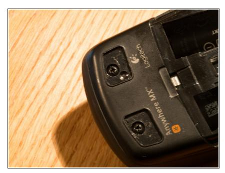
The front screws are underneath the front gliders. The can be removed with a butterknive or Plastic Opening Tool. The gliders have three layers, be careful not to seperate them.
