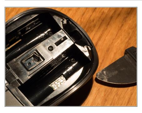
The back screws are underneath the stickers with the battery images.
