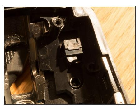
Put a piece of tape over the groove.
