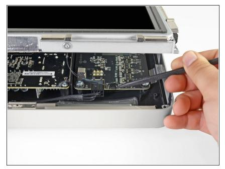
Disconnect the vertical sync cable in the upper left corner of the screen.
