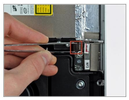
Grasp the SD board cable connector with a pair of tweezers and pull it straight away from its socket on the SD board.
