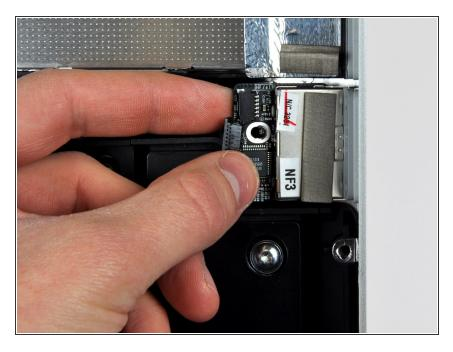
Lift the free end of the SD board to clear the plastic optical drive fan body, then pull it away from the edge of the outer case case to clear the two mounting pins.
