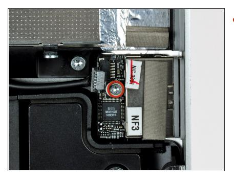
Remove the single T8 Torx screw securing the SD board to the outer case.
