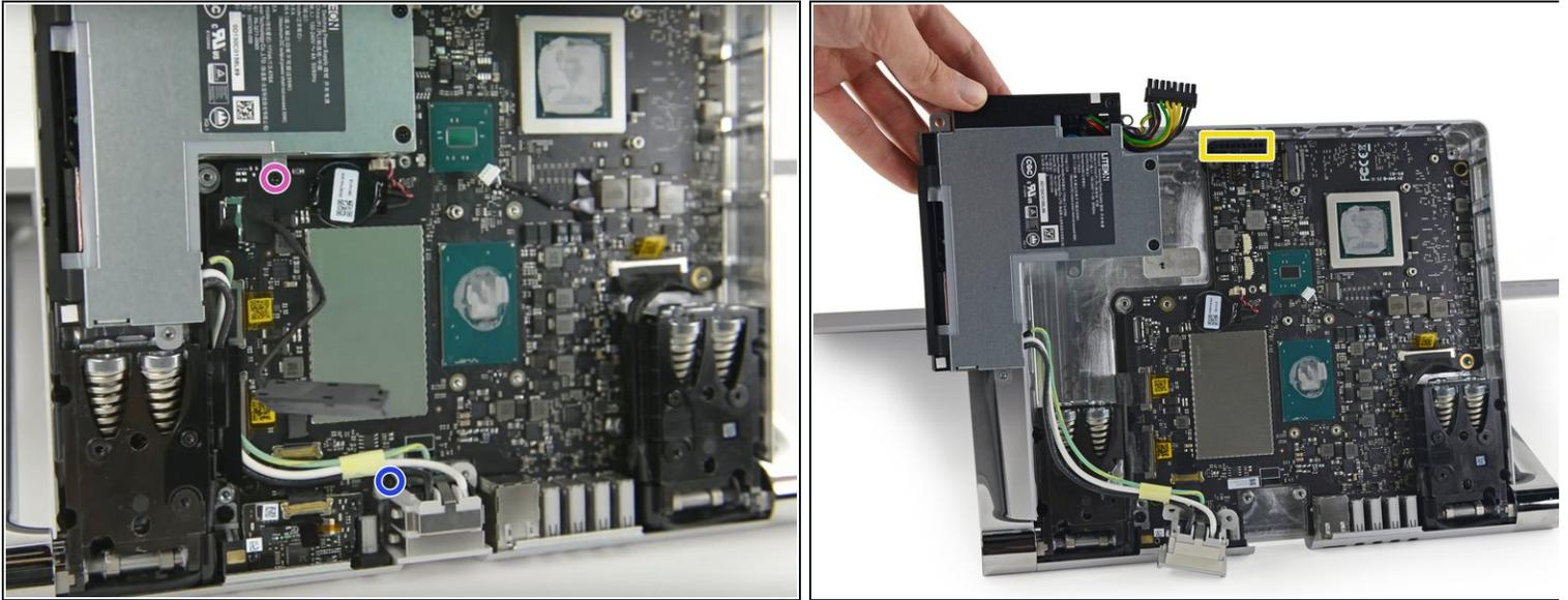
**i** Although removing the power supply is not necessary, it makes accessing the connectors easier
