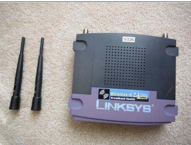
• Let's begin with the teardown! First, unscrew the antennas from the back of the router and set them aside.
