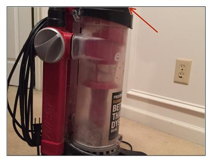
Flip the black release handle and remove the dust canister from the vacuum.
