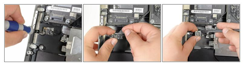
Remove the T8 Torx screw securing the Bluetooth board to the case.
