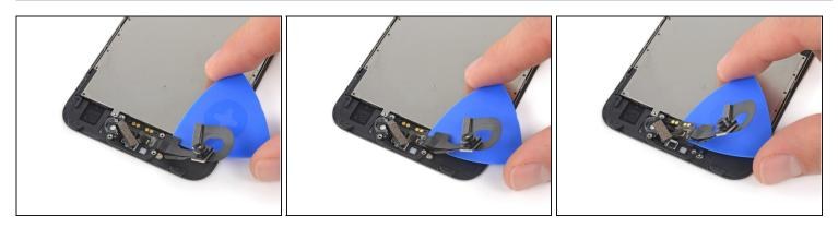
• Use the pick to lift the camera cable up off of the two plastic posts on the front panel and separate it from the last of the adhesive.
