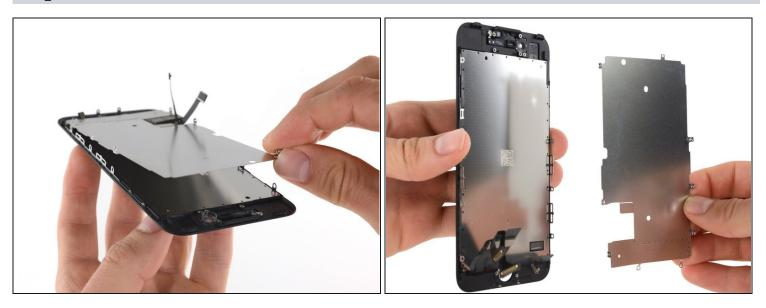
Gently lift the LCD shield plate from the display assembly.
