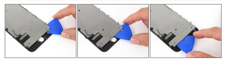
• Use an opening pick to break up the adhesive near the home button that holds the LCD shield plate to the display assembly.
