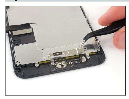
Remove the bracket that secures the home/Touch ID sensor.
