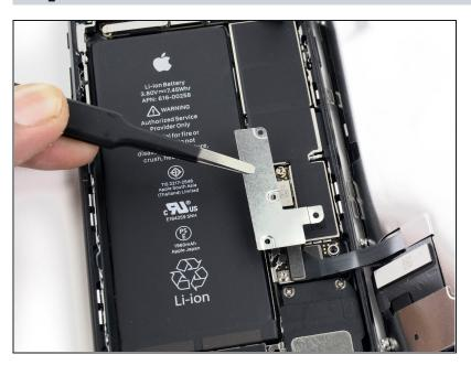
Remove the lower connector bracket.
