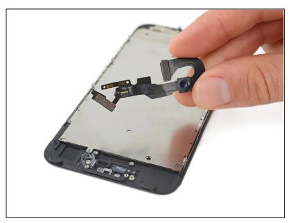
• Remove the front camera and sensor cable.
