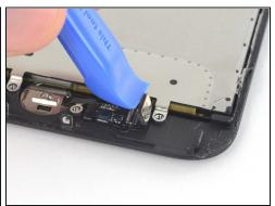
Pry under the left edge of the home button cable connector to disconnect it from its socket.
