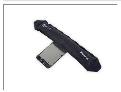
Heat an iOpener and lay it over the edge of the shield closest to the home button to soften the adhesive holding it in place.
