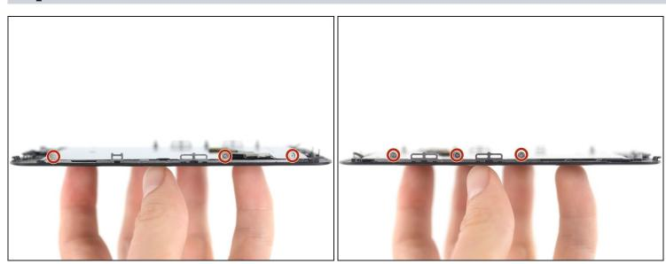
• Remove the three 1.2mm tri-point Y000 screws from either side of the display assembly for a total of six screws.
