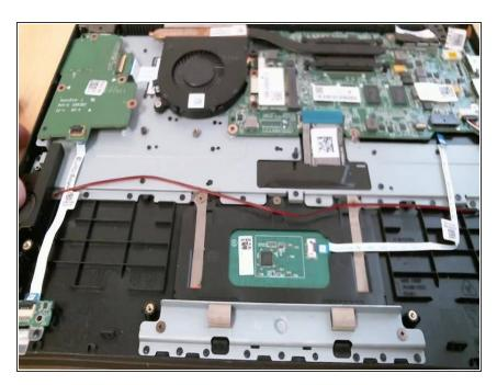
Start by lifting up the right hand side of the daughterboard so that it is removed at a slight angle. This is due to the SD card and the SD card port on the side of the palmrest.
