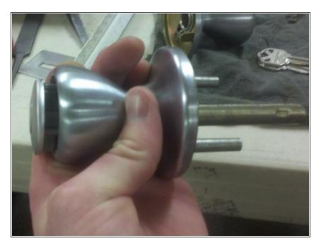
Gently pushing the end of the cylinder removal tool into the back of the lock should dislodge the cylinder from the rest of the lock.
