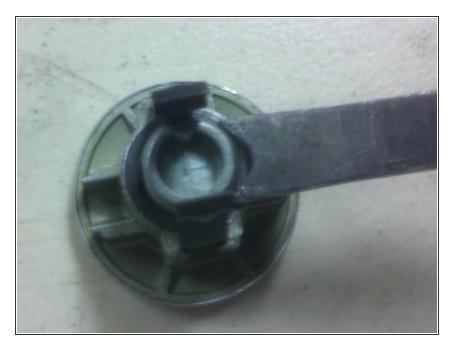
Use the forked end of the cylinder removal tool to remove the c-clip from the back of the plug.
