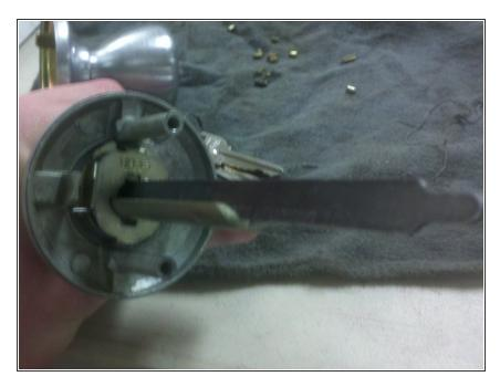
With the driver bar removed, insert the forked end of the cylinder removal tool into the back of the lock.
