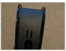
• Find the largest plastic seam on the side of the router and use the metal spudger to pop it out. There is no adhesive, though the snapping piece is relatively secure.
