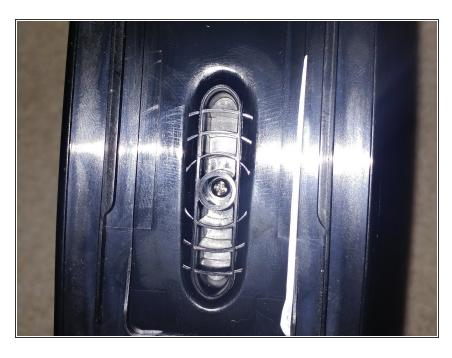
Remove the sticker from the bottom of the router and unscrew the base attachment. Once unscrewed, pull the base off of the main part of the router.
