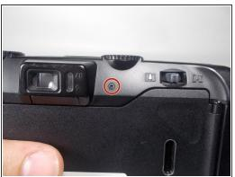
Using a Phillips J00 head remove the three 5mm screws on both left and right side of the camera as well as the one in back of it.
