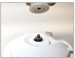
Whilst holding the fan on the inside, unscrew the silicon grip on the top of the blender. This should unscrew with a small amount of force.
