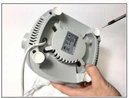
Remove the base of the blender by removing the 4 screws at underneath...
