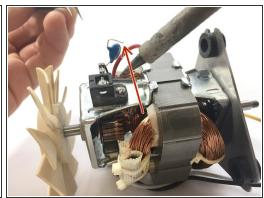
Using a soldering iron, heat up the solder attaching the capacitor to the side of the motor. This
