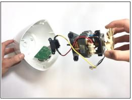
Unscrew the black box holding the safety switch next to where the motor attaches to the case. You
