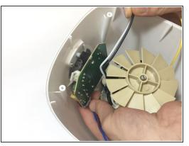
Detach any cables/wires from the switch panel. They should be attached with an easy to remove pinch clip (just pinch to unclip).
