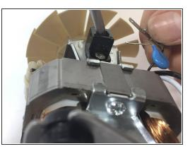
Using a little pressure, insert a 02 Phillips screw driver into the little black slot next to where you
