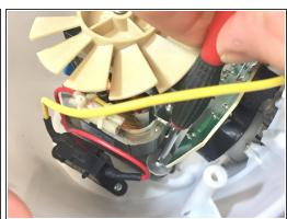
Unscrew the 3 screws attaching the motor to the top of the case.
