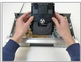
Remove the DVD tray assembly from the casing by lifting it up, sliding it back a little and tilting the back towards you as can be seen on the photos.
