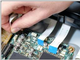
Remove the three ribbon style cables on the side of the DVD tray assembly by gently pulling them out of their slots on the board.
