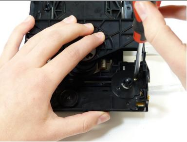
Unscrew the two 5mm screws that are securing the motor using the #1 Phillips screwdriver.
