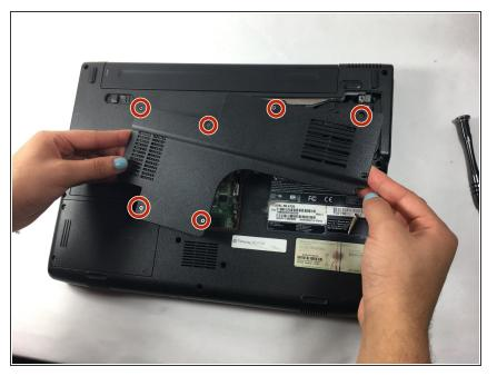
Remove the six screws with the Phillips #0 Screwdriver that secures the middle large piece of the back panel.
