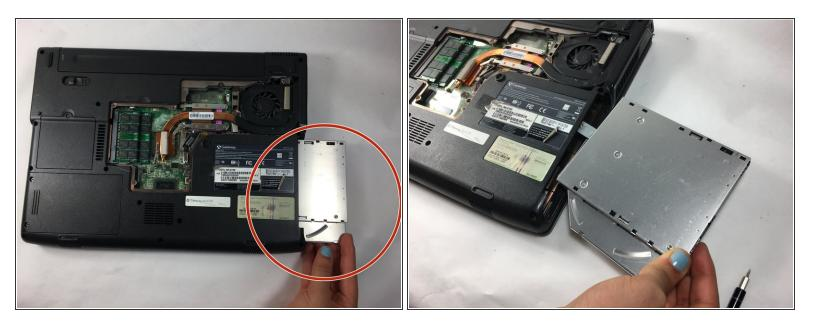
• With that screw removed, you can now pull the disc drive out of the laptop by pulling on it in the direction that it slides.
