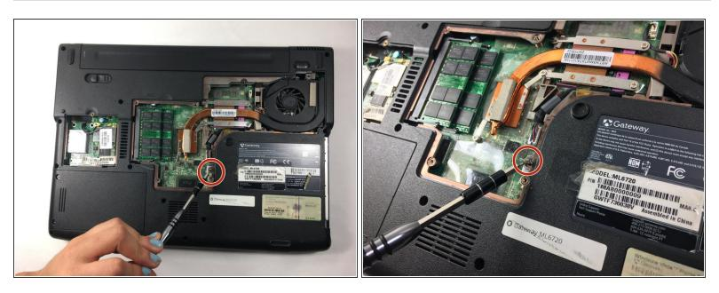
Check to see if your laptop requires a screw(s) to be removed for the disc drive. Remove the screw (s) holding the disc drive down.
