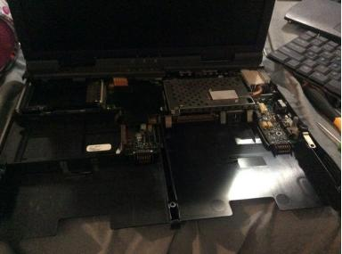
Disconnect the cables and pull out the top base orange connector and the keyboard blue connector then you can remove both the keyboard and the top base
