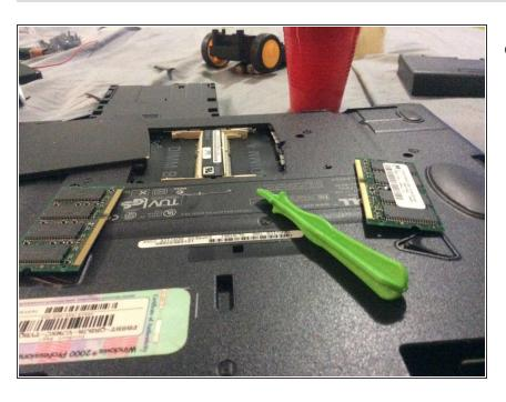
Use the green tool to remove the ram compartment cover then remove the ram.
