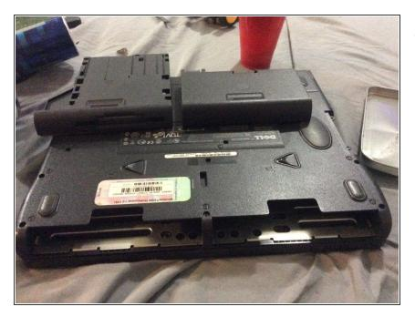
Push the triangle things and hold them there with one hand and take the battery out and do the same to the cd drive you can get all the tools for this guide from a iPhone disassembley kit
