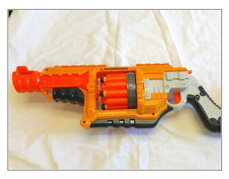
Reattach the other plastic half of the gun. Tighten the screws and you're done.
