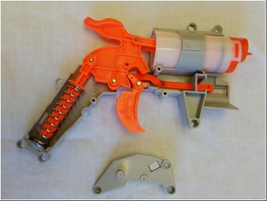
• Remove the three screws holding the trigger plate in place, then remove the plate carefully.
