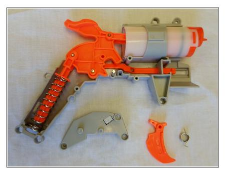
Remove the spring and trigger mechanism from the gun and set aside.
