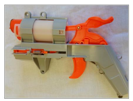
Remove the exterior spring from the sliding mechanism and rotate the gun to the opposite side.
