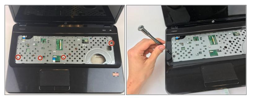
• Remove the four 7.25mm screws located by the red markers.
