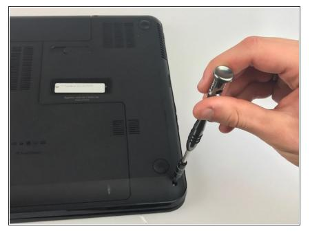
• Flip the laptop over and remove six 7.25mm screws.
