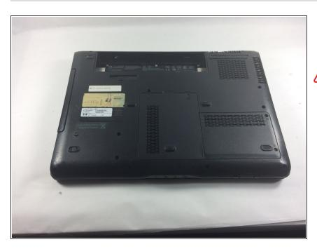
• Remove the battery by sliding the button to the side.
