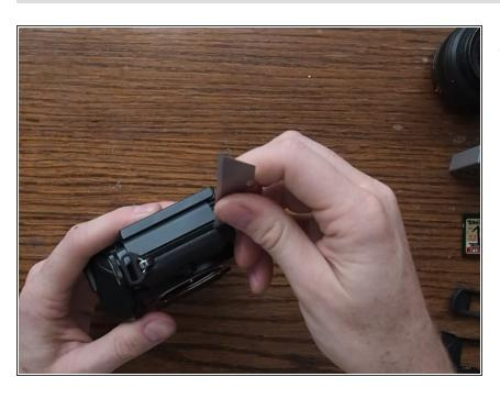
Use the utility knife to pull the rubber covers from the front of the camera.
