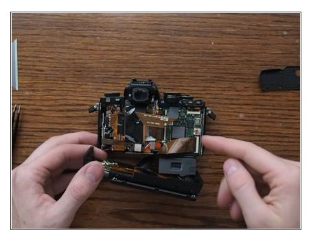
Lift the tiny black flap that holds the ribbon cable for the LCD to the camera body. This releases the ribbon, you shouldn't need to pull on the ribbon with any force.
