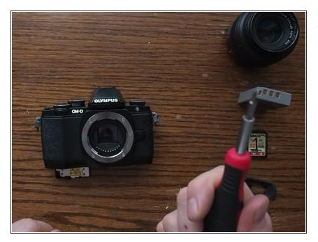
Unscrew all the screws you can find on the outside of the camera, except those on the lens mount and those on the LCD itself. Watch the video for a rundown of each screw location.
