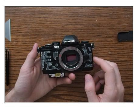
Remove the screws from the front of the camera. (not the ones on the silver lens mount)
