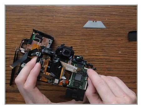
If you want to remove the top plate, you will need to release this ribbon cable, as well as remove two screws on the sides next to the camera strap connection points.
