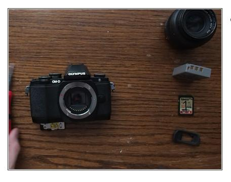
Remove the lens, battery, SD Card, and EVF eye cup
