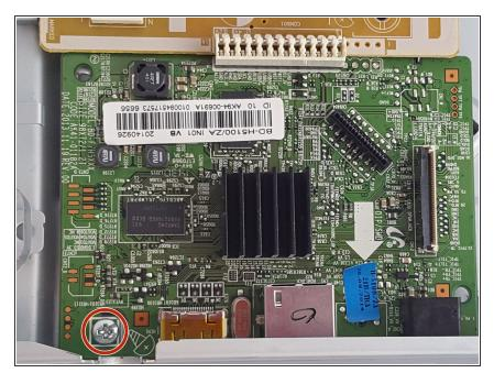
• Use a Phillips Head #2 to remove the 7.5mm screw.
