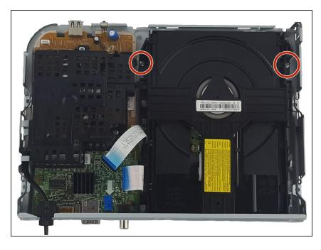
Remove the two 7.5mm screws on both sides of the disk tray with Phillips Head #2 screwdriver.
