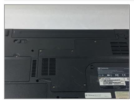
Locate the battery at the very top on the backside of the laptop.
