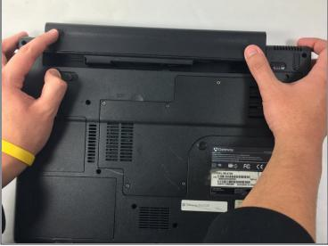
• With both latches unlocked you can now slide out the battery, by pushing it off the top.
