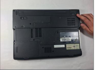
• Slide the latch in the top right corner to the right, to set it to unlocked.
