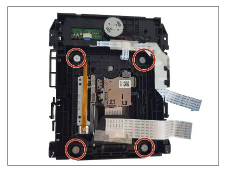
Use the Phillips Head #00 screwdriver to remove the four 6.2 mm corner screws.
