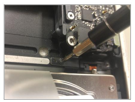
Using PH00 bit, unscrew the 4mm Phillips screw holding down the ribbon attaching the HDD to the motherboard.
