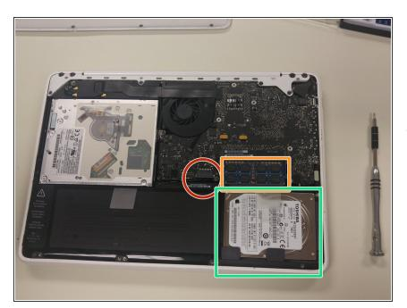
Identify the parts we need to remove. Start with unplugging the battery (circled in red), followed by
