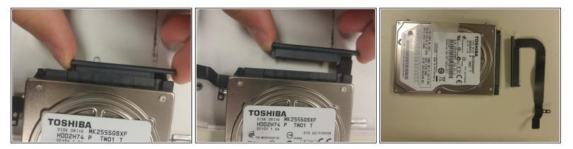
Remove the SATA cable from the hard drive by gently pulling the connector away from the body of the hard drive.
