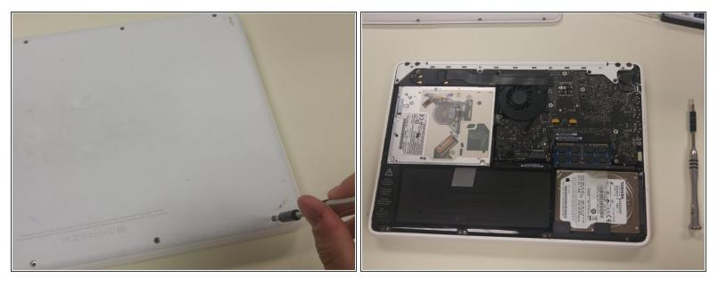
● Using a PH00 bit, remove the eight 4 mm Phillips screws securing the lower case to the MacBook.
