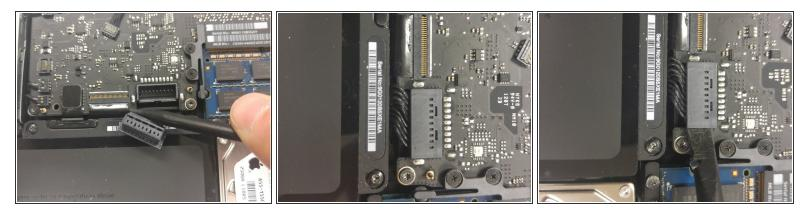
• Use the flat end of a spudger to lift the battery connector up out of its socket on the logic board.
