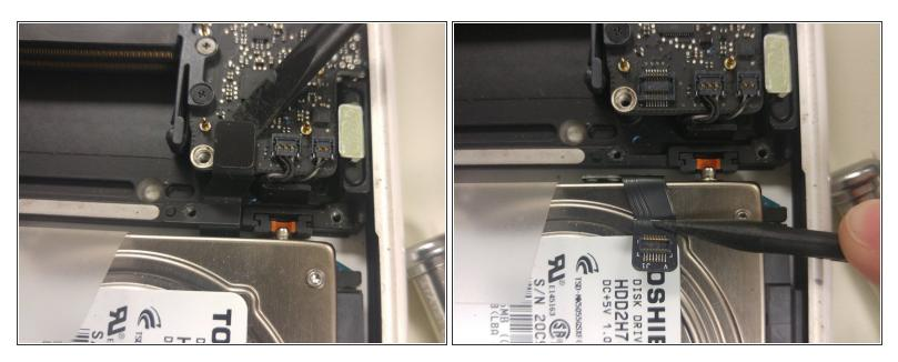
• Using the flat end of a spudger, detach the ribbon from the motherboard.
