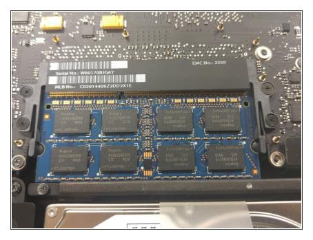
Release the tabs on each side of the chip by simultaneously pushing each tab away from the RAM.
