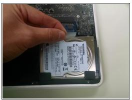
Once battery is unplugged, remove two Philips head screws using J00 bit.
