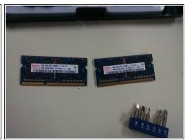
Locate the RAM Directly above the Hard Drive. Gently push the two snaps away from the RAM cards and gently pull the ram out. You Will do this step again to remove the Second card beneath the first.
