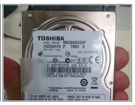
After removing the screws and plastic cover piece, remove the hard drive then unplug from Logic Board.
