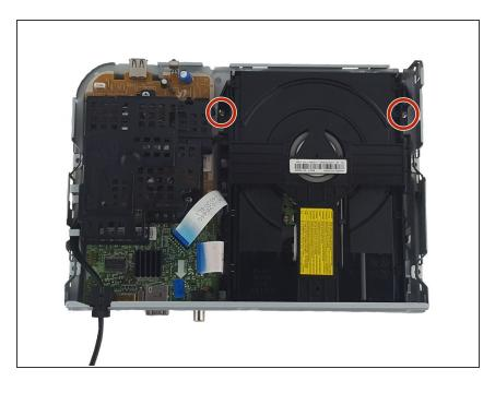
Remove the two 7.5 screws on both sides of the disk tray with Phillips Head #2 screwdriver.
