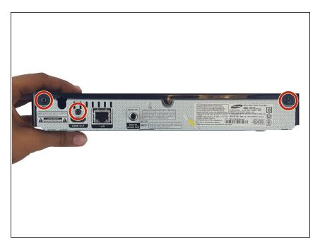
Use the Phillips Head #2 screwdriver to remove the three 10mm screws on the back panel.
