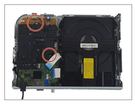
Use a Phillips Head #2 to remove the two 7.5mm screws on the black cover.
