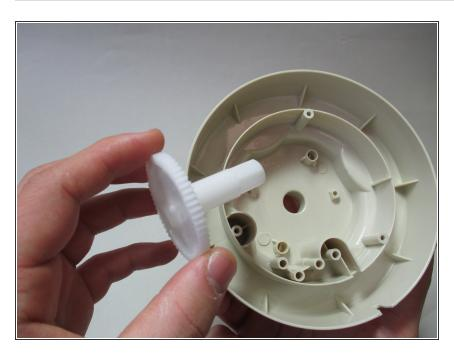
Remove the gear from the bottom casing.
