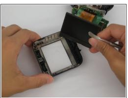
Use the metal spudger to remove screen from device.
