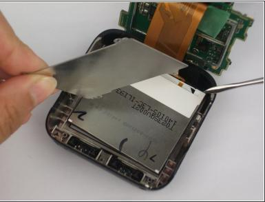
• Use the metal spudger to remove metal plate from device. This will reveal the screen.
