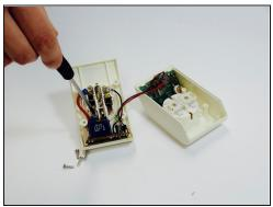
• Use the #1 Phillips head screwdriver to remove the screws on the inside.
