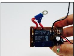
• Pull the PCB (printed circuit board) from the case.
