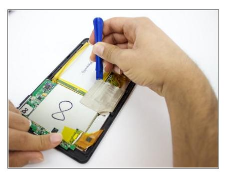
Lift the edge of the white tape with the iFixit opening tool.
