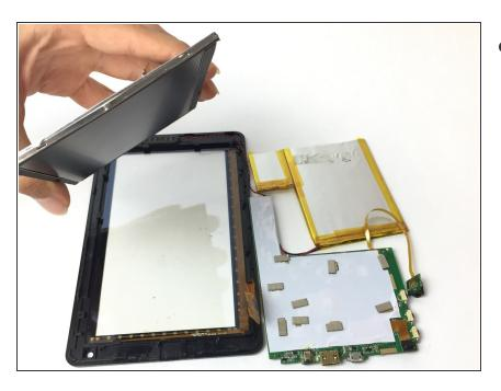
Using your fingers, remove the defective screen from your device.
