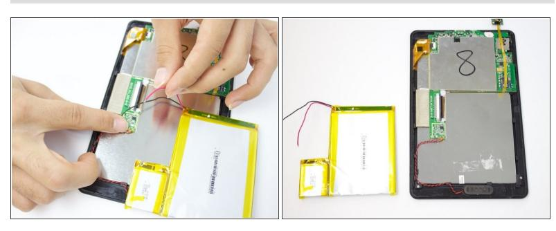
Remove the two wires. Then remove the battery completely from the device.
