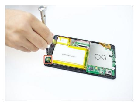
On the bottom of your tablet, use the Phillips #0 screwdriver to take the two 3mm screws out.
