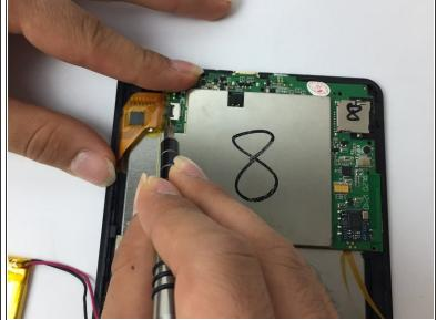
Locate the orange connection strip that connects the motherboard to the display screen. Use your J001 to pry the connector off.
