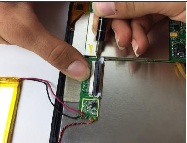
Take your J001 screwdriver and carefully push out the cable ribbon alternating on both sides.
