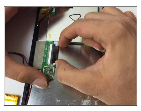
After you loosened the cable ribbon with your J001 screwdriver, pull it out with your fingers.
