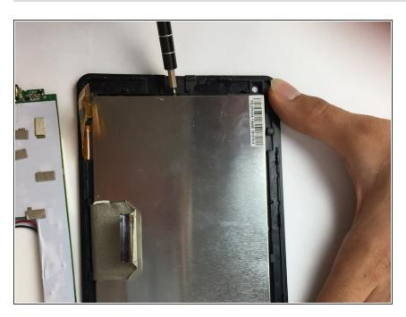
Pry off the display screen using J001 screwdriver.
