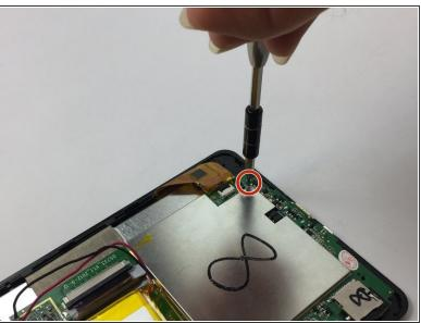
On the bottom of your tablet, take your J000 screwdriver and take out the three 3mm screws that hold down the motherboard.
