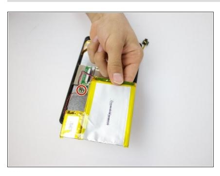
Lift the battery and place it a little further away from the positive and negative battery wires.
