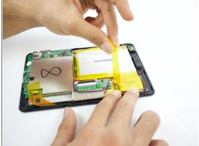
• Lift the white tape with your fingers, then lift the yellow tape that holds the battery extension.
