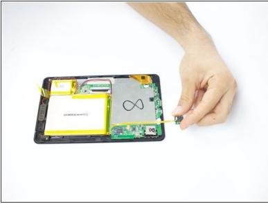
• Lift the headphone jack and move it to the other side, placing it on the surface you are working on.
