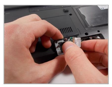
Separate the Bluetooth adapter by pulling it from its casing.
