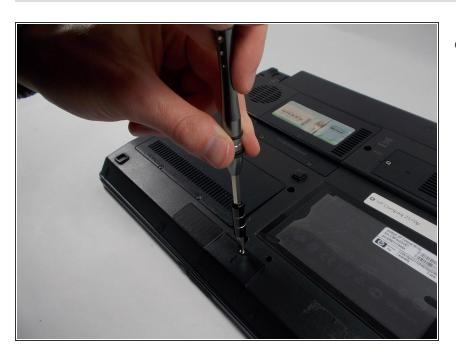
There is 1 screw on the panel you located in step one. Use your Philips head screwdriver to remove the single screw.
