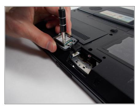
Pull the adapter to the left exposing its underside. Locate and remove its only screw using your Phillip's head screwdriver.
