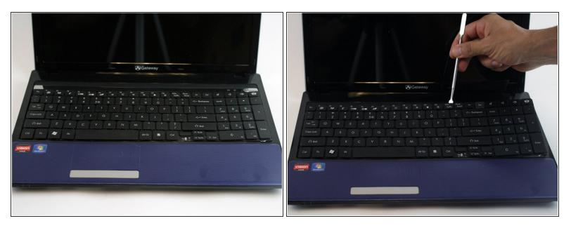
• Locate the top of the keyboard, then insert a spudger into the top most edge of the keyboard where it meets the bezel surrounding it.
