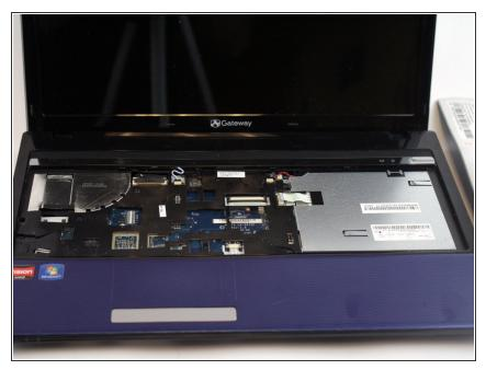
Using the spudger, lift the keyboard from its base to expose the underside components.
