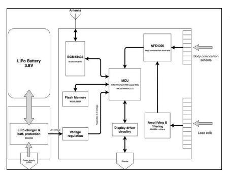
I've made an attempt to design a block diagram for the whole setup. This won't be 100% accurate as I don't know all the details but it will give you an idea on how the components are interlinked and work together.
