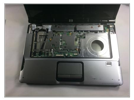
Insert new keyboard by sliding it into place of original keyboard and clipping into place near top of trackpad.
