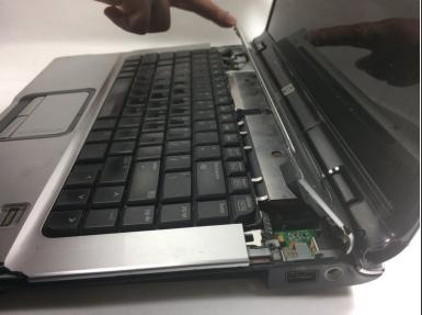
Gently lift the plastic panel on the top of the laptop at the divide until the two ribbon cables and cable leads are visible with their ports on left side on laptop.
