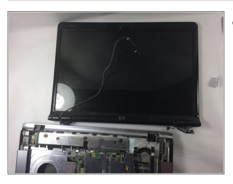
Feed the cables through the laptop and lift the monitor from the rest of the computer.
