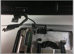
• Remove the four 7mm screws holding screen to keyboard, there are 2 on each side.
