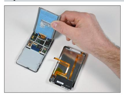
The front and back of the iPod should now be completely separated.
