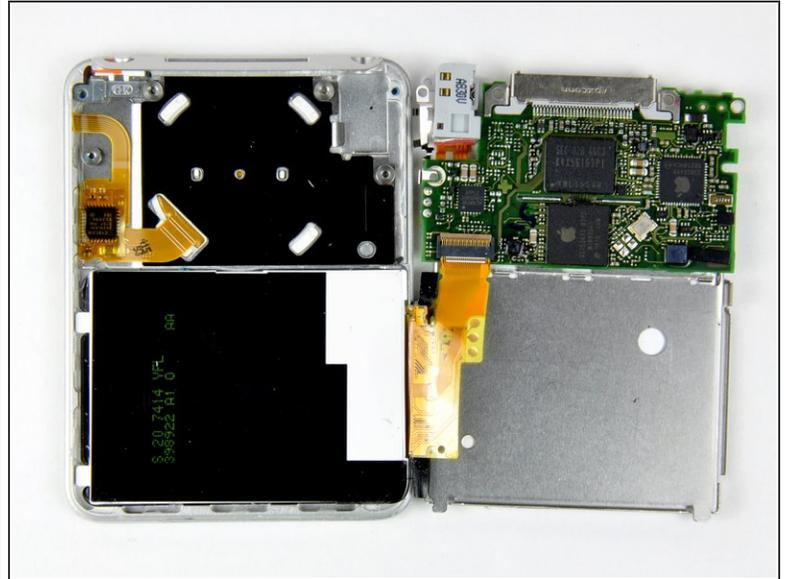
**⚠** The logic board is still connected to the front case by the display ribbon cable, located on the headphone jack side of the logic board.
