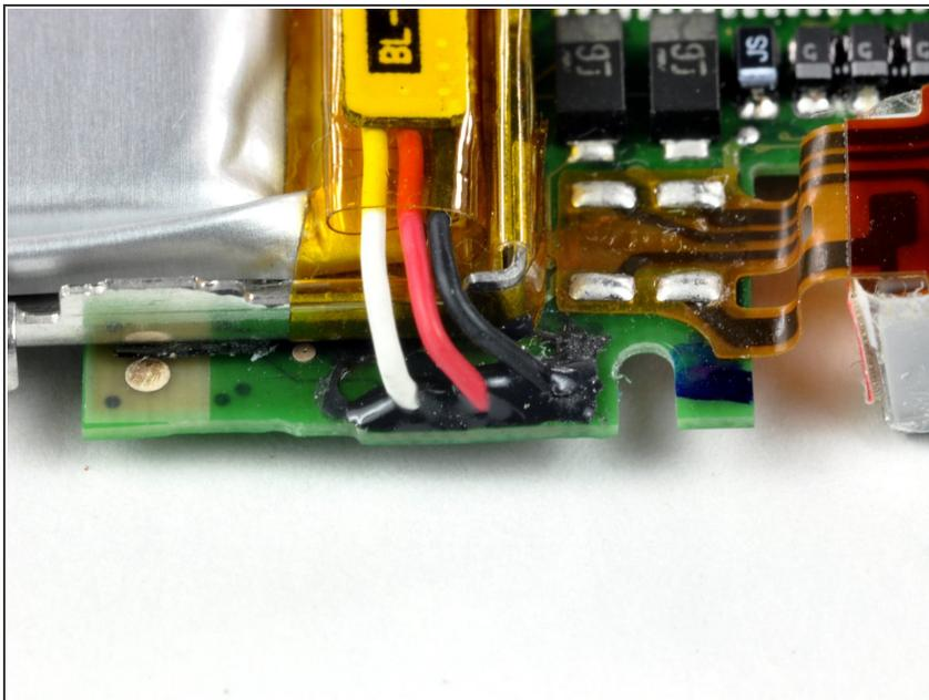
**⚠ Battery replacement on the iPod Nano 3rd Generation requires soldering. Before proceeding, be sure you have all the required tools and a general feel for soldering small electronic components.**
